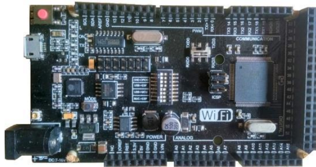
Figure 3. Arduino microcontroller ATmega2560 R3 Wi-Fi.
